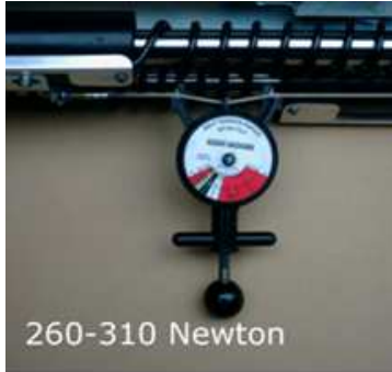
Figure 1.28: Measuring cable tension
