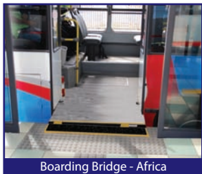
Boarding Bridge - Africa
