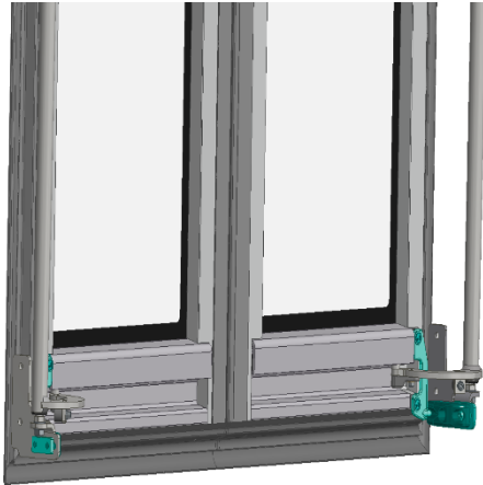
Figure 22: Catch wedge and catch block locations
