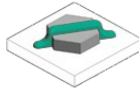
Figure 2: Fastener marked with a torque marker
